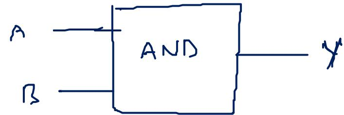
→ entity describes the inputs and output ports of a logic module & provides external view of component.
